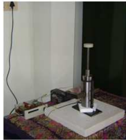
Fig. 4 The complete damper unit
